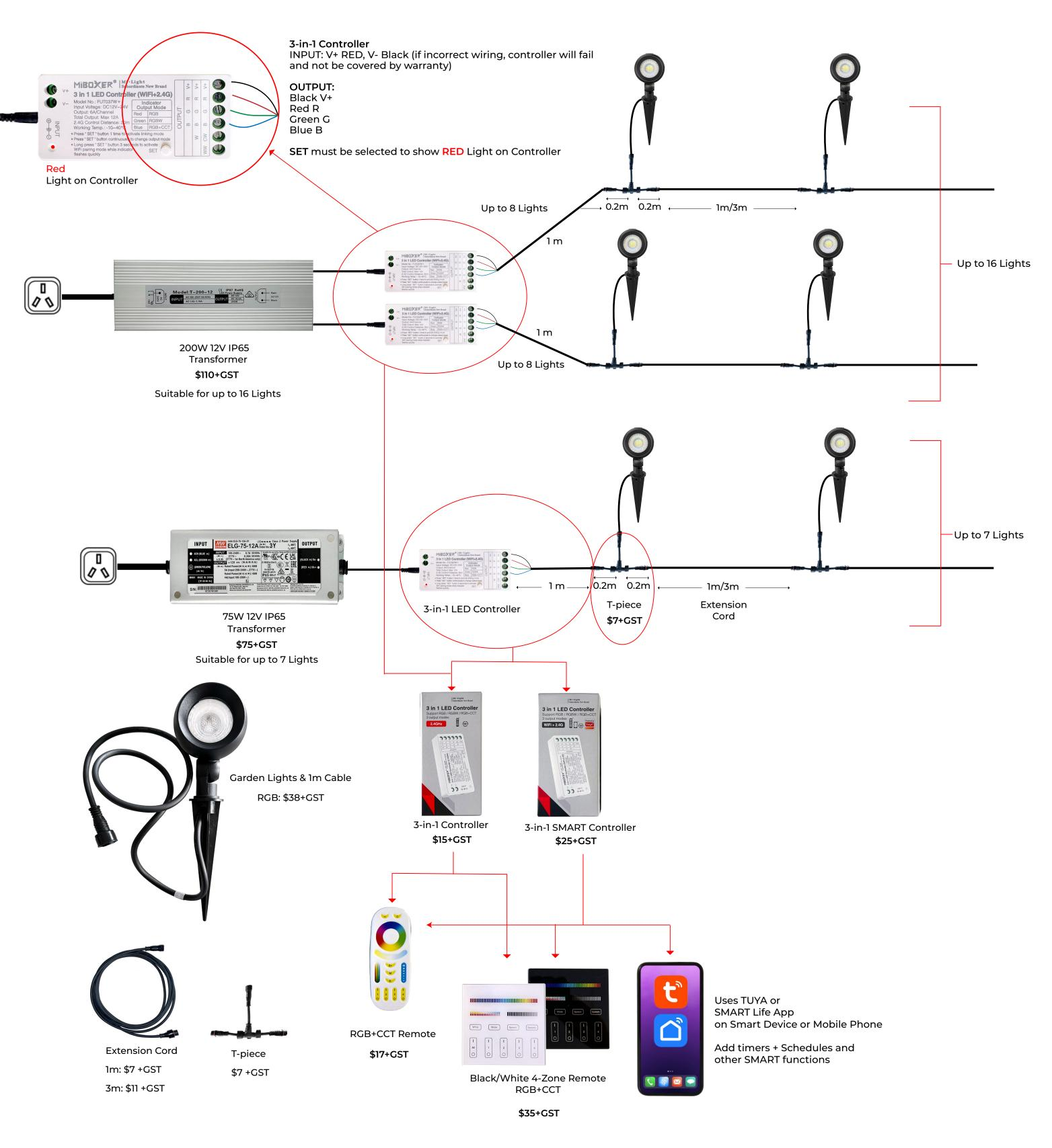
NB: To ensure long life, use silicon when connecting connectors. Please note that connectors can get old with time and water can damage cables and connections.
